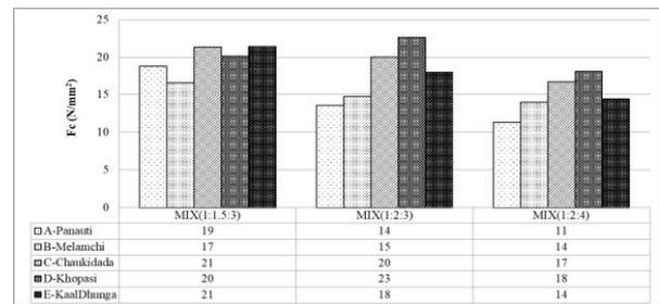
Fig. 7 Cube compressive strength (28 days) with various mix ratio and aggregate type
