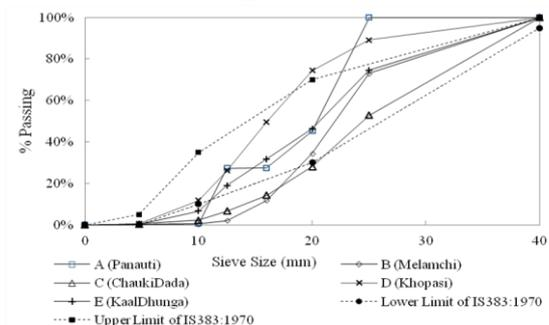
Fig. 4 Aggregate gradation showing upper and lower limits of IS383:1970
