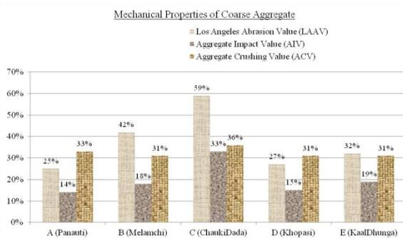
Fig. 5 Mechanical properties of coarse aggregates
