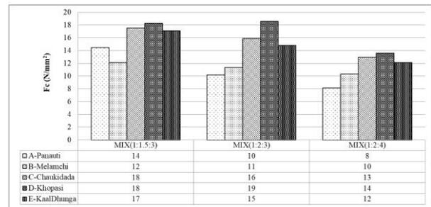
Fig. 6 Cube compressive strength (7 days) with various mix ratio and aggregate type
