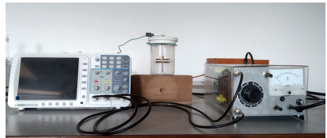
Figure 2. Experimental set-up of the disc electrode system, which produced discharge using high voltage and high-frequency power supply at atmospheric pressure.
