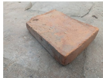
Figure 5. Sample of burnt clay brick used in study
