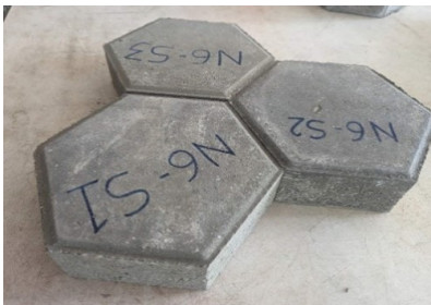
Figure 3. Impermeable blocks of 60 mm height
