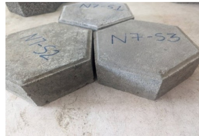
Figure 4. Impermeable blocks of 70 mm height
