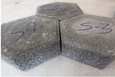
Figure 2. Permeable blocks of 70 mm height
